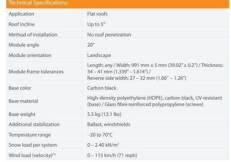
Allowed frame width on the reverse side of the module
